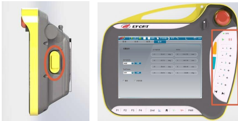
Figure 4-9 hand pressing and function key of teaching pendant at right side
