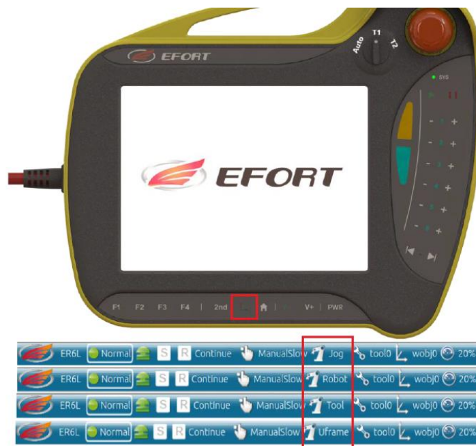
Figure 4-8 switching of coordinate system
