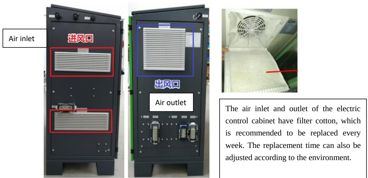
Figure 3-2: cleaning of filter cotton at air inlet and outlet
